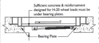
Products utilizing steel or aluminum are typically referred to as fabricated doors. These doors transfer the applied load through beams to bearing plates on each end. Unlike cast iron, these bearing plates are not designed to adequately support the design loads. This area may require additional reinforcement and concrete support to transfer the design load.
