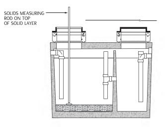
3.) Measure the height of the solids. If the height of the solids and grease are greater than 25 percent of the liquid depth then the interceptor needs pumping.
